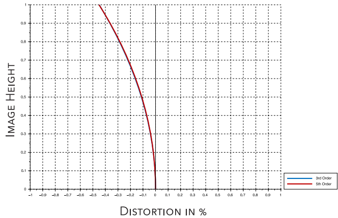
IMAGE HEIGHT VS. DISTORTION
