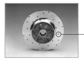
Laser welding on 46SV impeller: spot welding follows impeller blades all along the profile
