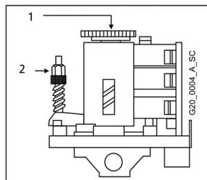
Adjustment of the differential pressure determines the start pressure P.
