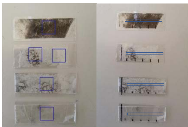
Figure 2 Examples, how the measuring field areas ( 1\text{cm}^2 ) can be set on the adhesive tape samples and the influence of the result using the square centimeter as a square or a line.
