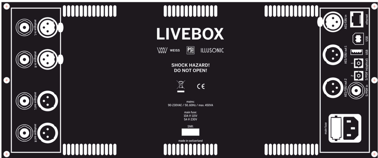
Rear panel of the LIVEBOX with USB, AES/EBU and S/PDIF inputs, analog connections, and a network port.
