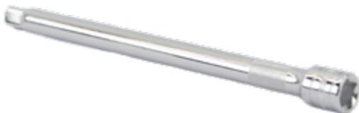
1/2" Drive Extension | MT-TK-EX-00-2-UNI Material: Heat treated chrome vanadium steel Finish: Chrome plated Size: 10" Long (1.75" x 12.25" x .75")
