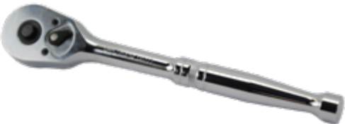
1/2" Drive Quick Release Oval Head Ratchet | MT-TK-RT-00-2-UNI Material: Heat treated chrome vanadium steel Finish: Chrome plated mirror polish Size: Handle 7.5" Long (2.3" x 11.5" x 1.5")
