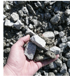
Crushed aggregate mineral sub-base
