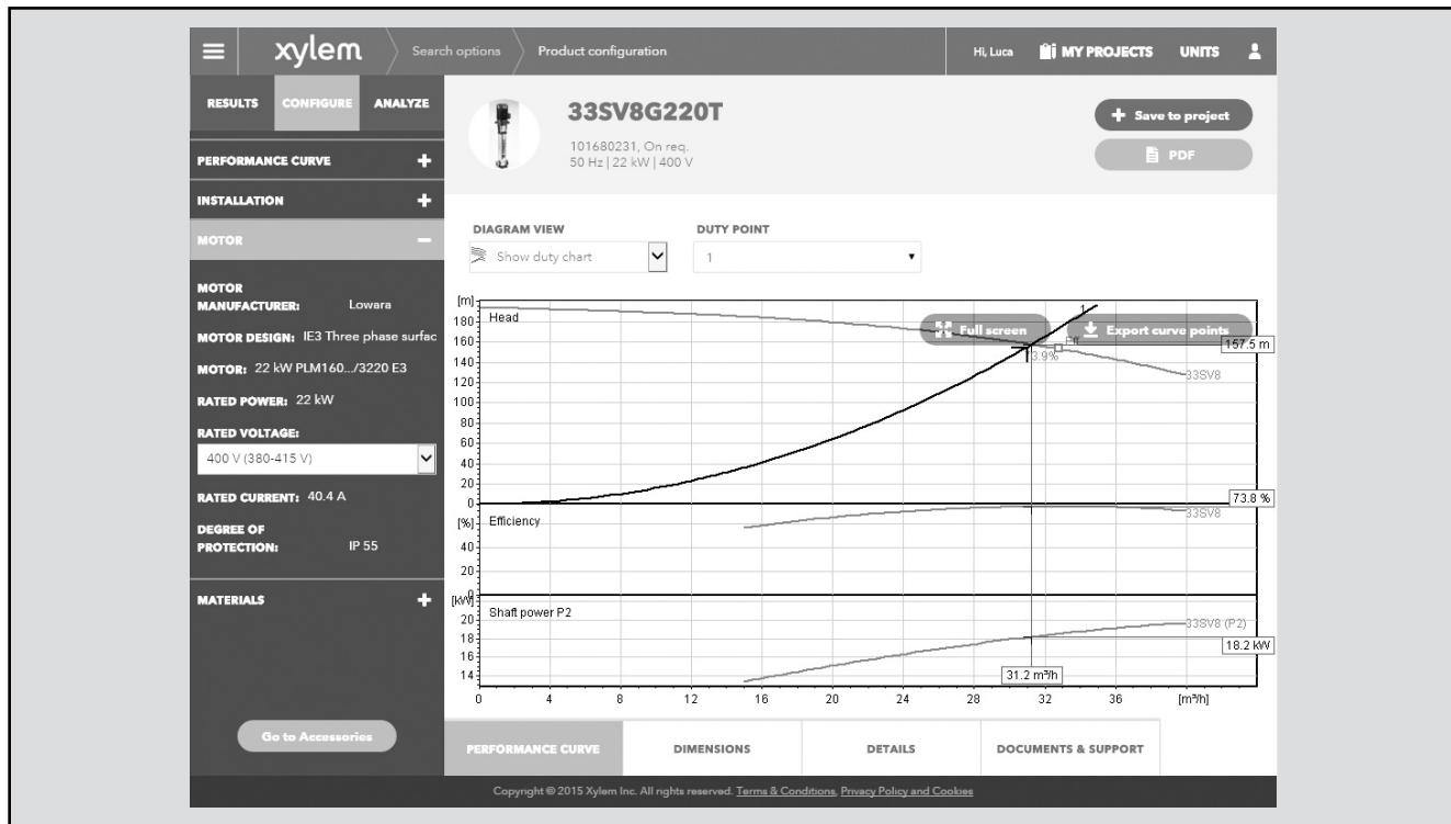
The detailed output makes it easy to select the optimal electric pump from the given alternatives.
